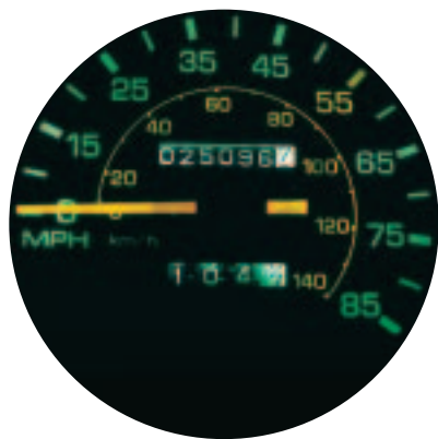
Figure 4 The speed shown on the speedometer gives the instantaneous speed—the speed at one instant in time.
