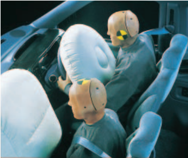
Figure 20 These crash dummies were restrained safely with safety belts in this low-speed crash. Usually humans would have fewer injuries if they were restrained safely during an accident.
